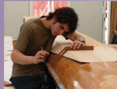
The work of building new masts and spars for Hispania, Blue-Bird, Dirdam, Giradilla and other mast repairs made it necessary to build a mast shed for our shipwrights. The shed is equipped with work benches and a mast building bench that is long enough to build and repair any kind of wooden mast. We store a large quantity of spruce which is known to be the ideal wood for masts and spars and which enables us to do any repair in a short space of time.
