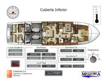
Integrated control and alarm systems have revolutionized life on board over the last decade. Historical alarm logs or tank and bilge level records, which were logged by hand, are now registered and stored automatically, in formats which can be later presented by means of tables with personalized filters, sorted according to their relevance or in easy to read graphics.
