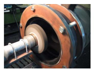
**Corrosion** might appear on sterntubes (mostly on aluminium ones) especially on the area of bearing housing and on the seals. This corrosion can be repaired by welding should the necessary means be available for its further machining.
