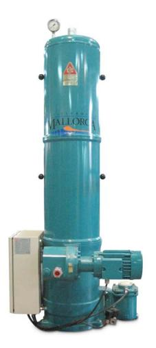
Astilleros de Mallorca offers a filtering and separating service for fuel oil. Our separator removes water by coalescence and at the same time minimizes oil contamination levels of particles and oil degradation products (oxidation resin/sludge, varnish) by means of a fine filtration. The system has a filtration degree of 3 microns absolute.
